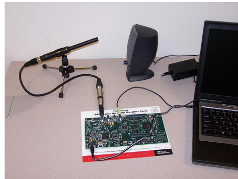
Fig. 2. The DSP-based prototype for real-time one-way communication
