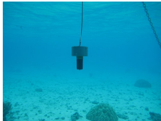
Figure 1: Test 2 transducer set-up. Photo depicts receiver transducer suspended from the boat in about 3 meters water depth in the Viapahu Lagoon
