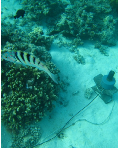
Figure 2: Test 4 transducer set-up. Photo depicts receiver transducer placed on the bottom of the Viapahu Lagoon in the ‘bommie field’ at about 2 meters water depth
